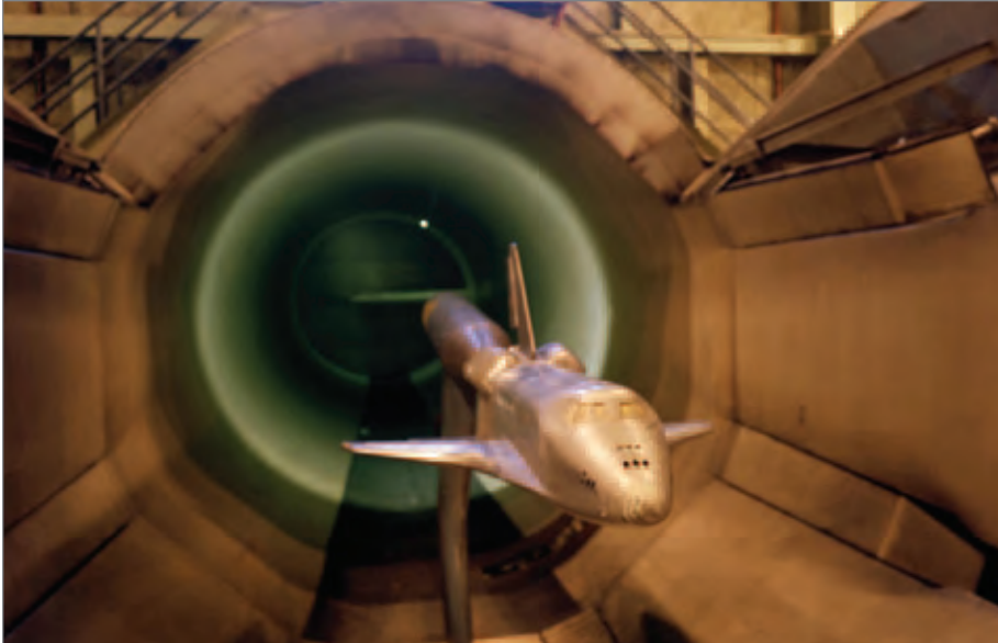
A model of the Space Shuttle in the 16-foot Transonic Wind Tunnel at NASA Langley Flight Research Center.
