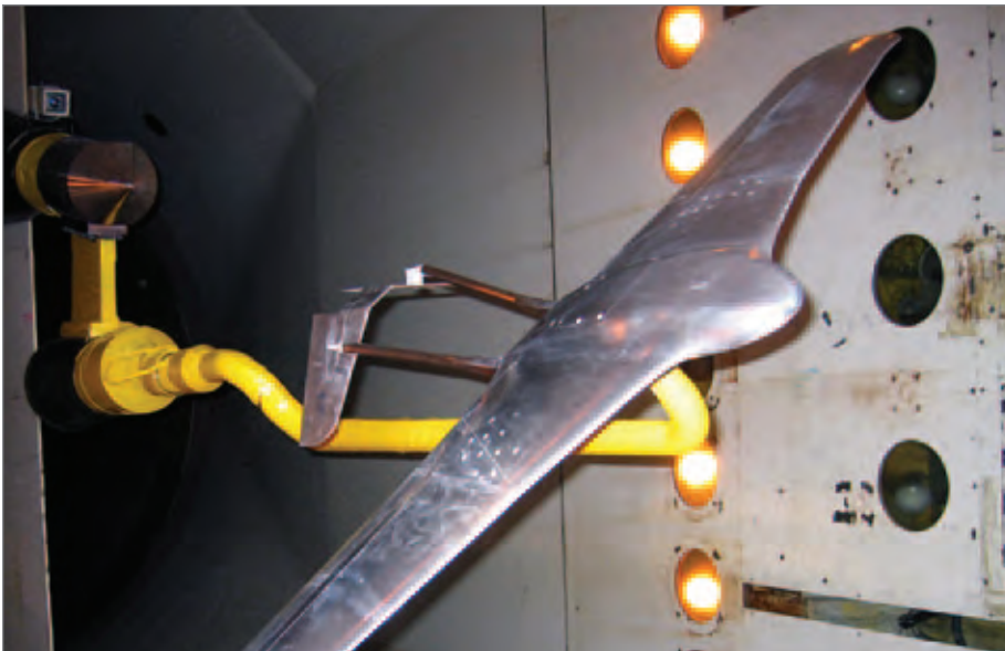
A scale model of the ARES being tested in the Langley Research Center Transonic Dynamic Tunnel. This model has the wings and tail in their fully developed positions.
