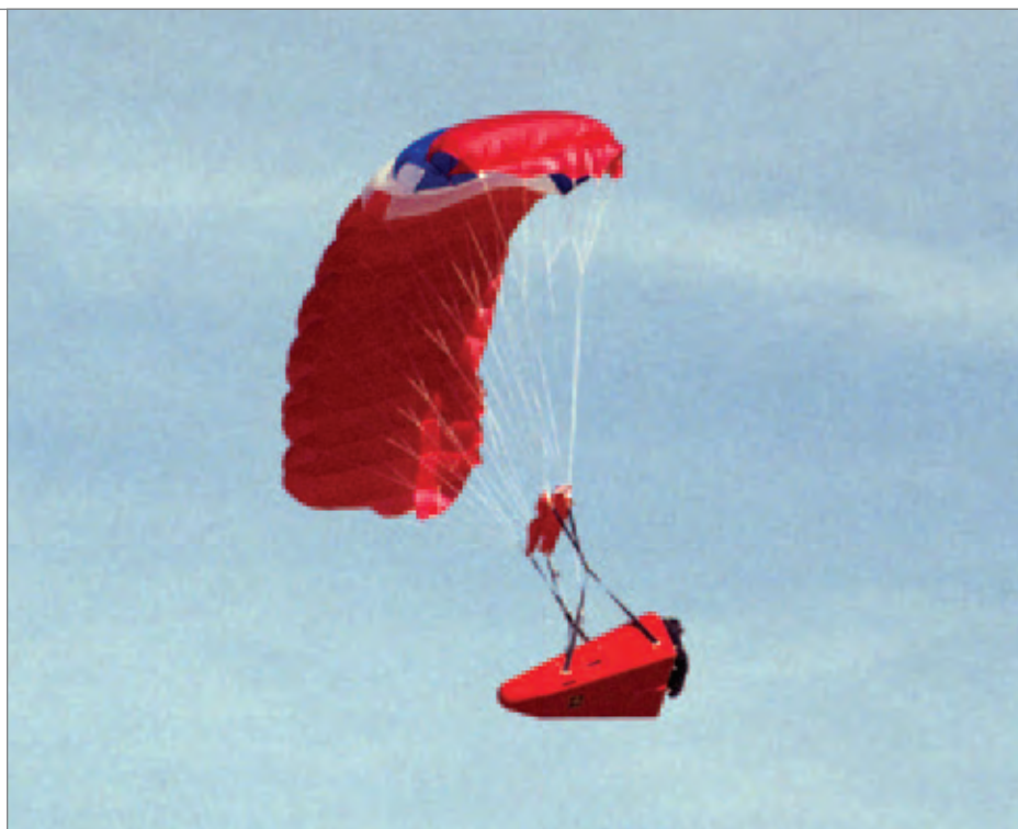
One of the Spacewedge remotely piloted research vehicles in flight under a steerable parafoil during 1995 research flights conducted by NASA's Dryden Flight Research Center.
