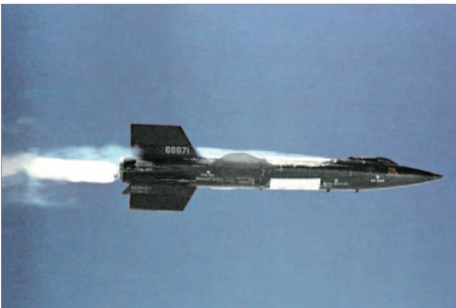
The X-15 #2 (56-6671) launches away from the B-52 mothership with its rocket engine ignited. The white patches near the middle of the ship are frost from the liquid oxygen used in the propulsion system to cool the payload bay, cockpit, windshields, and nose.
