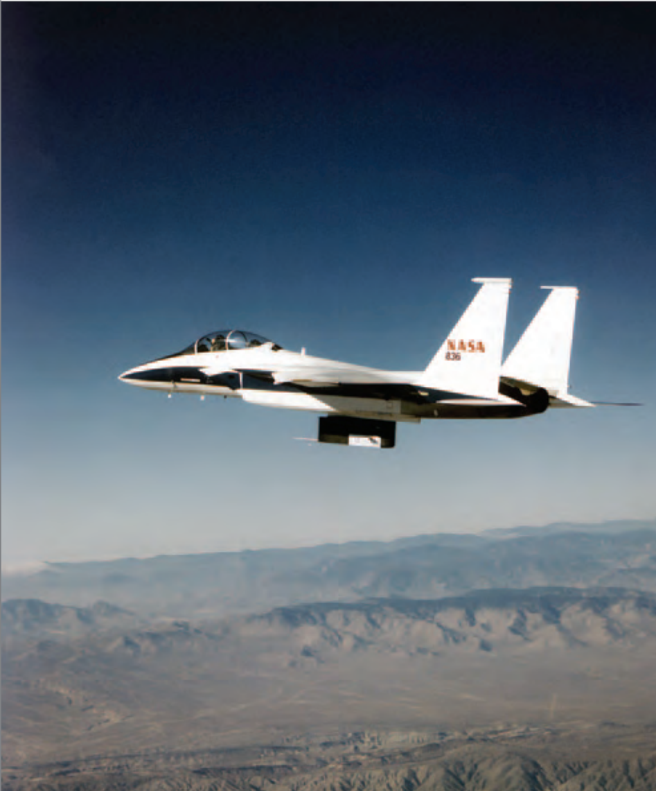
F-15B testbed in flight with new sonic shockwave sensor.
